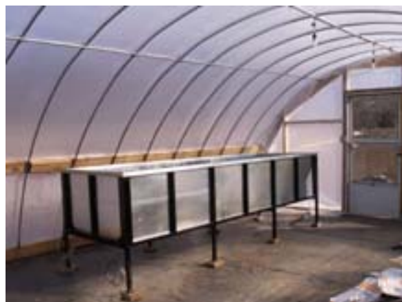
Piedmont Biofarms' vermi flow-through digester contains 100 lbs. of red wiggler worms that consume about 50 lbs. of food per day.
