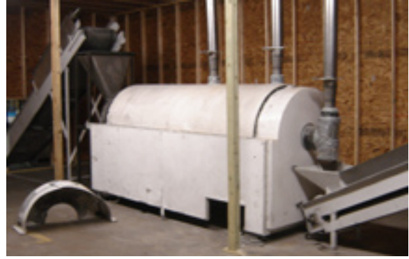
Dry scrubbers on Metech’s glass processing line remove CRT coatings and crush the glass, resulting in a cleaner product and valuable commodity.
