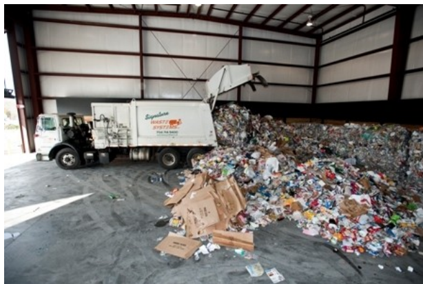
A collection vehicle unloads single-stream recyclables on the Sonoco tipping floor.
