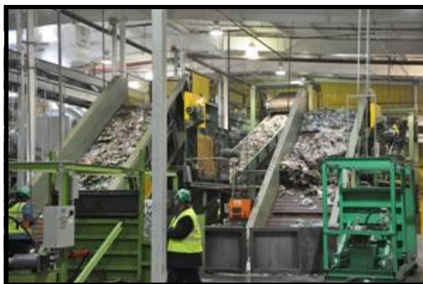
Employees operate machinery and equipment at the initial in-feed of PET bottles in the Clear Path recycling plant.
