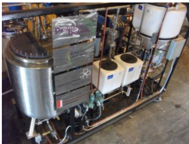
Piedmont Biofuel's new enzymatic biodiesel plant, seen here, expands the range of feedstock — fats, oils and greases — able to be produced into B100-grade biofuel.
