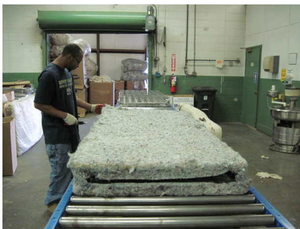
Mattress Go Round TM employee (above) removes old cotton padding from the metal innerspring frame.
