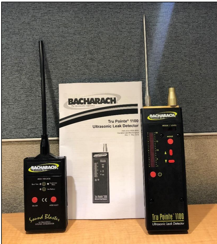
SoundBlaster Ultrasonic leak detector and Tru Pointe 1100 ultrasonic leak detector along with the Instruction Manual
