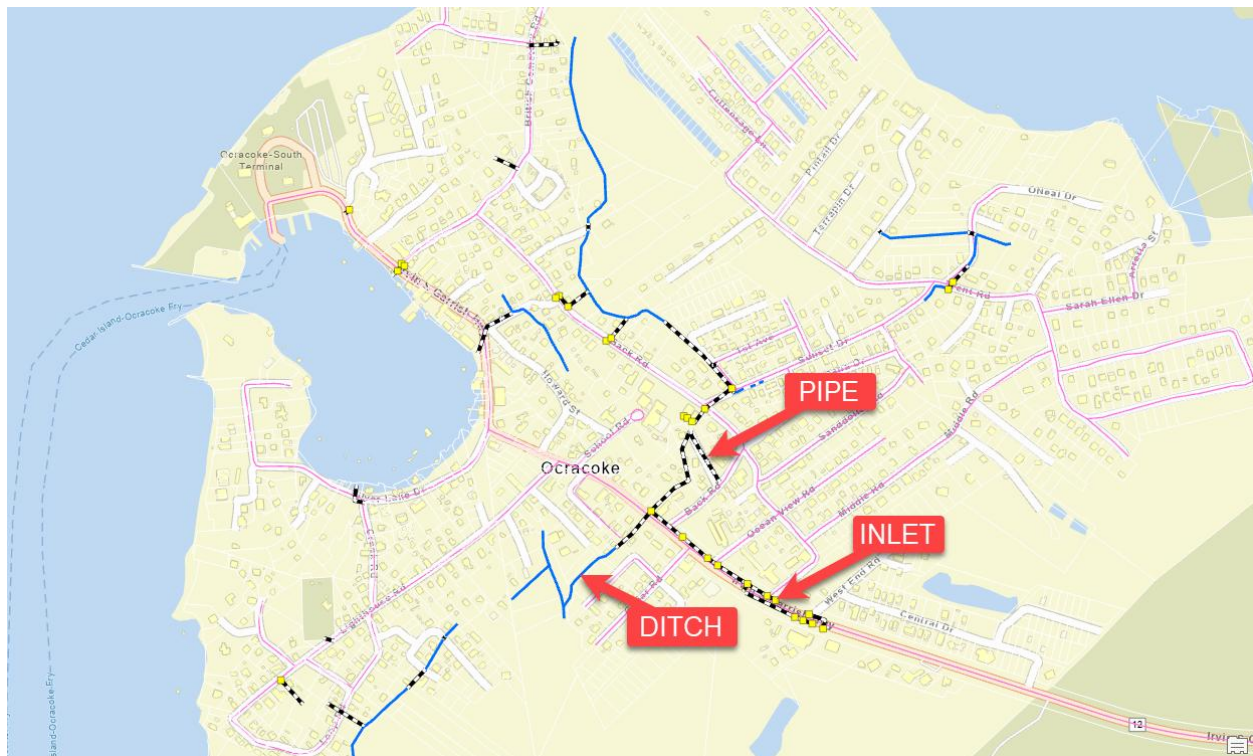
Figure 20: Approximate Drainage Mapping Completed During RCCP
