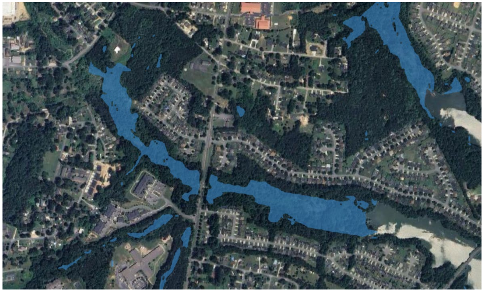
Figure 5. Finalized Vector Wetland Layer Created by WetAMP Tool (Blue Polygons are Predicted Wetlands)
