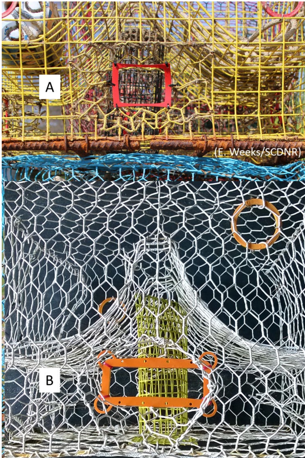
Figure 4.5.10. Premade plastic diamondback terrapin excluder devices shown inside one entrance funnel opening of crab pots. (A) The “SC design” shell width limiting excluder. (B) A shell height limiting excluder.
