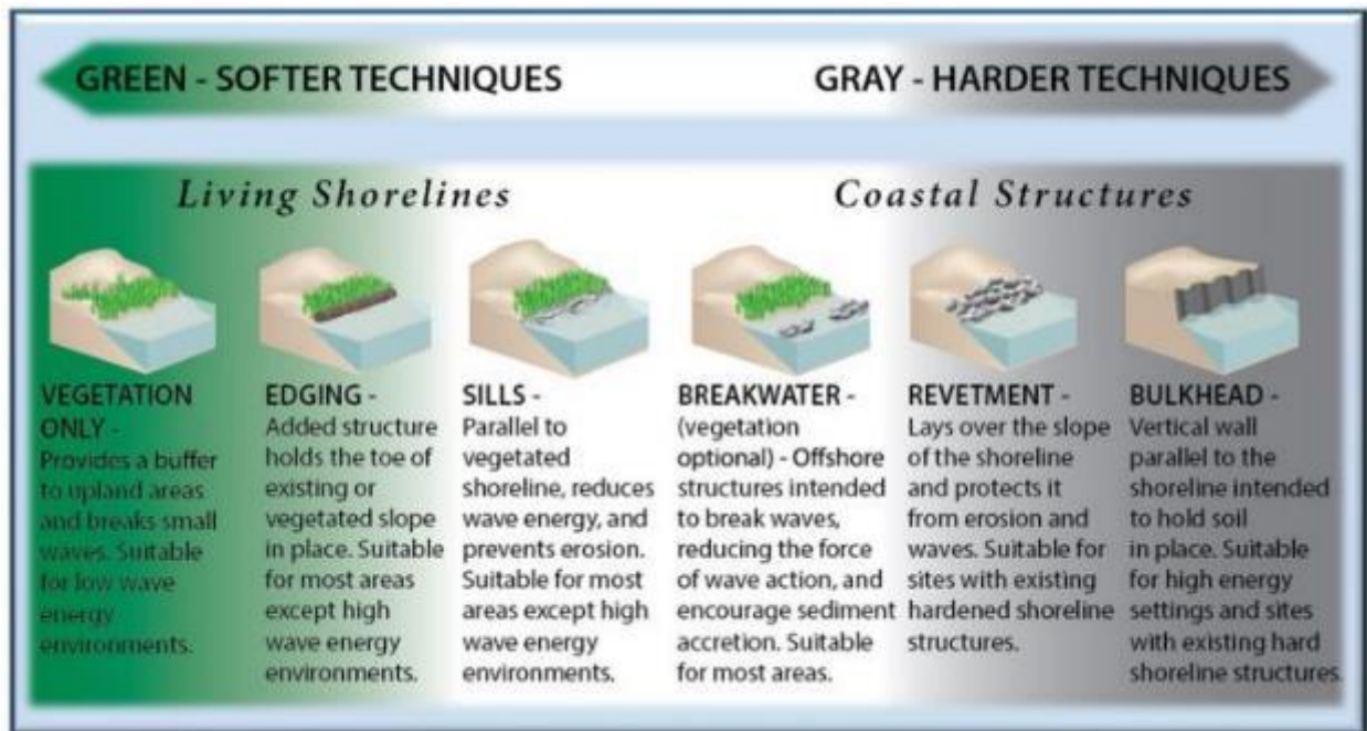
Figure 5.7. Continuum of shoreline stabilization methods, from most natural and softest (green) to least natural and hardest (gray), with the greenest methods being more effective in low to moderate wave energy, and grayest methods being more effective for high wave energy. 105
