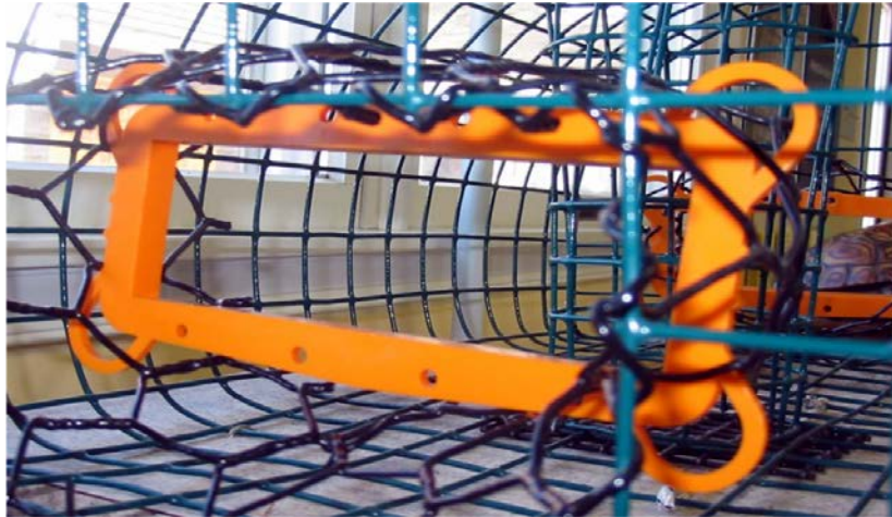
Terrapin excluder device on a commercial crab pot. (Wetlands Institute 2010)
