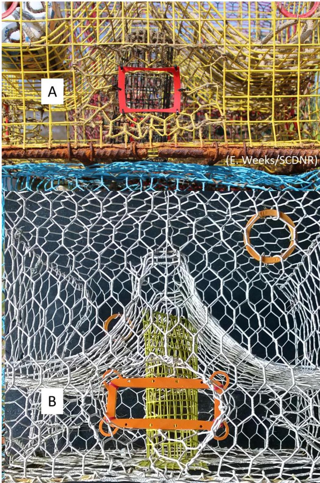
Figure 4.5.3. Premade plastic diamondback terrapin excluder devices shown inside one entrance funnel opening of crab pots. (A) The “SC design” shell width limiting excluder. (B) A shell height limiting excluder.
