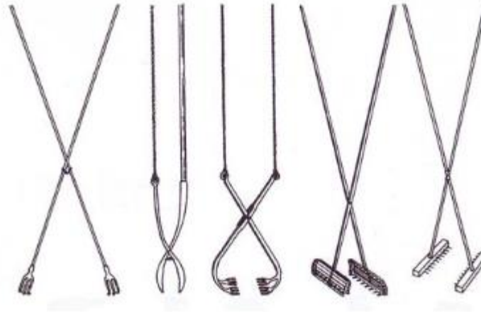
Figure 8. An illustration of several different designs for hand tongs and rakes that may be used for harvesting oysters (from Shafi 2007, reproduced from von Brandt 1964).
