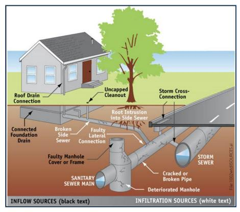
Figure 7.1. Example of inflow and infiltration (I & I) pathways.<sup>2</sup>
