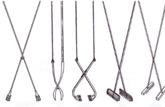
Figure 7. An illustration of several different designs for hand tongs and rakes that may be used for harvesting oysters (from Shafi 2007, reproduced from von Brandt 1964).
