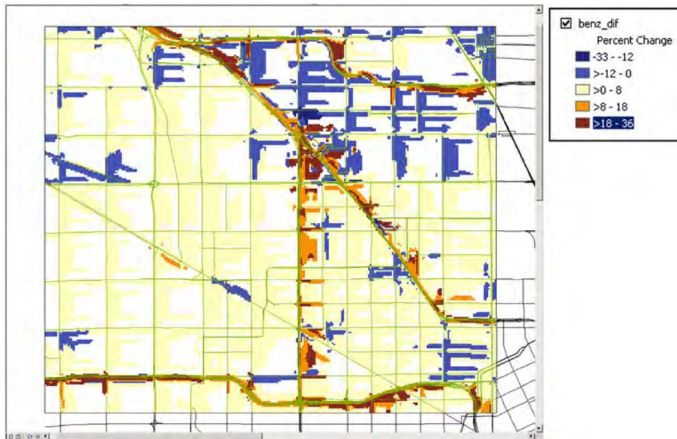
Fig. 5. Example of benzene concentration percent differences when VMT is increased by 20% and overall speed by 10%.
