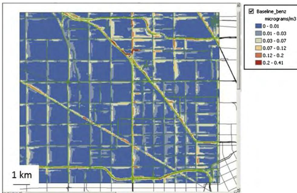
**Fig. 4.** Example of C-LINE model results: benzene concentrations ( $\mu\text{g}/\text{m}^3$ ) out to 500 m from each roadway segment.
