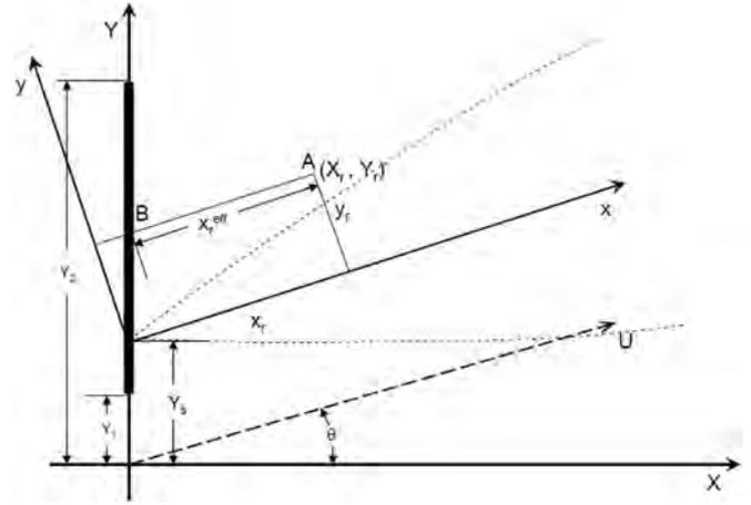
Fig. 1. Coordinate system used to calculate contribution of the point source at  $Y_s$  to concentrations at  $(X_r, Y_r)$ . The system  $x$ - $y$  has the  $x$ -axis along the mean wind direction, which is at an angle  $\theta$  to the fixed  $X$  axis. The dotted lines represent the plume originating from an elemental point source at  $(0, Y_s)$ .
