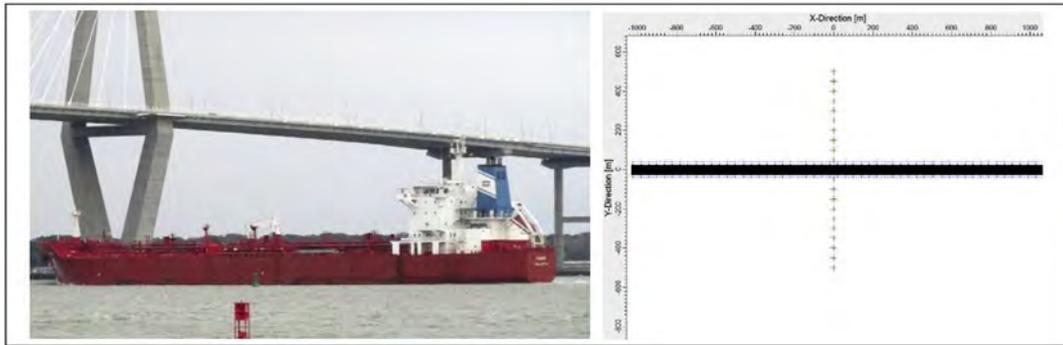
Fig. 3. Emission from ships in transit represented by buoyant line sources.
