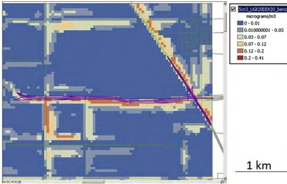
Fig. 7. Example of modeled benzene concentrations ( $\mu\text{g}/\text{m}^3$ ) for selected road segments as a base case scenario using unaltered input data.
