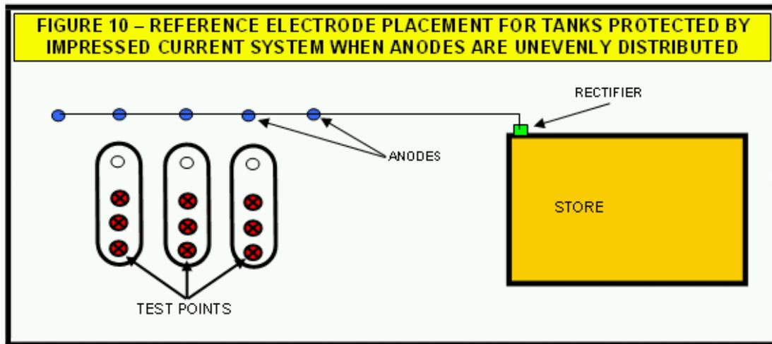
If it is not known where the anodes are installed, at least three measurements are required along the centerline of the tank. Testing should be conducted at as many locations along the centerline of the tank as are available. If soil access is available at each end of the tank and in the middle, all three structure-to-soil potentials should be recorded. If any one of the measured potentials does not meet one of the acceptable criteria, the structure should be failed.
