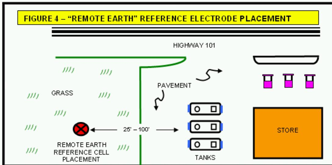
Care must be taken that the remote location is not in proximity to any other cathodically protected structure (e.g., natural gas lines) or directly over any other kind of buried metallic structure. The remote placement should be such that the reference electrode is aligned with the longitudinal axis of the tanks and can “see” the anodes. This orientation is desirable in order to prevent shielding.
