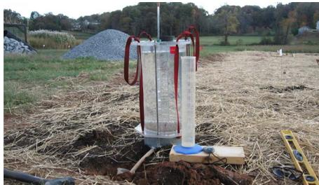
Figure 1. Cornell Sprinkle Infiltrometer used to make infiltration measurements.
