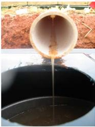
Figure 2. Storm water running off a compacted plot during a storm event.
