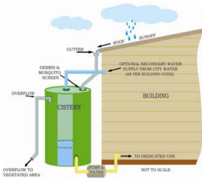
Figure 25-1. Typical RWH System (NCSU-BAE)
