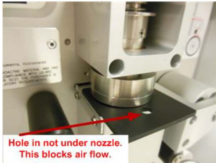
Figure 79. Leak Isolation Shim Position for Lower System Leak Test.
