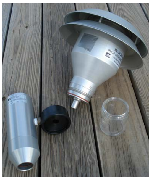
Figure 56. The PM10 Inlet Components.
