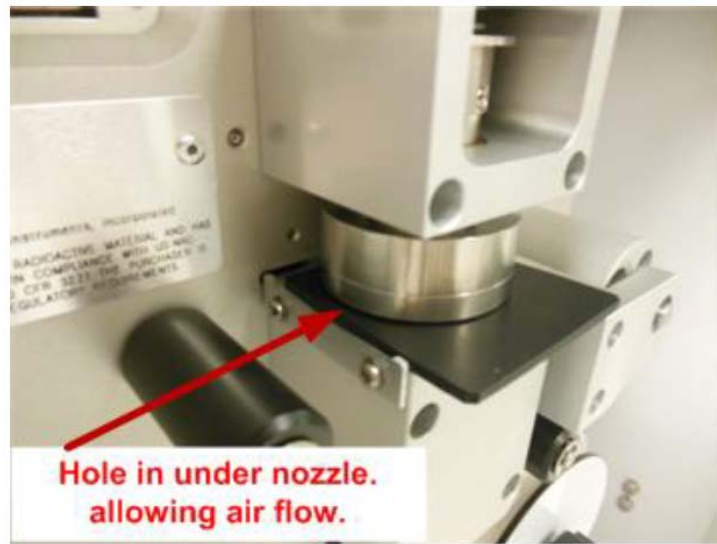
Figure 80. Leak Isolation Shim Position for Upper System Leak Test.
