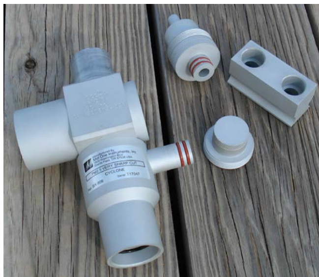
Figure 58. Disassembling the VSCC for Cleaning.
