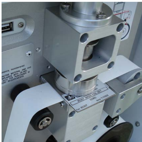
Figure 49. Proper Zero Foil Placement.
