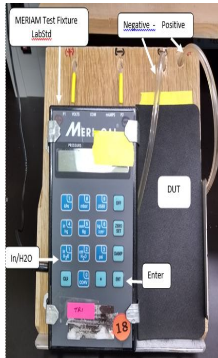
Figure 5. Meriam Lab Standard and DUT Setup.
