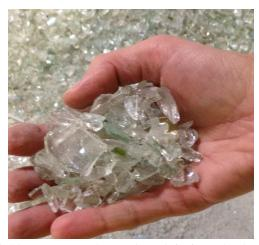
Glass-containing material, primarily from MRF operations, is fed by conveyor (shown above left) from the tipping floor into the plant. Clean, furnace-ready cullet is the final goal. Above right shows flint ready for the glass plant.
