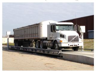
A dump trailer waits on the scales before proceeding to the tip floor to dump its load of glass.
