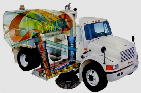
Regenerative air cleaners are the second most common. They work by directing air at a high velocity within a confined box the rides across the pavement. The uplift from the high velocity effectively loosens dust and other fine particles on and near the pavement surface and lifts them into a hopper at the back of the truck. This equipment removes surface-deposited sediments from all pavement types. This equipment is recommended for regular preventive maintenance.
