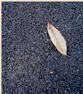
PA is like conventional (impervious) asphalt except that less fine material is used in the mixture to provide for drainage, resulting in has a coarser appearance than conventional asphalt. A modified asphalt binder as specified by the Carolina Asphalt Pavement Association (CAPA) shall be used to ensure long term durability and permeability.
