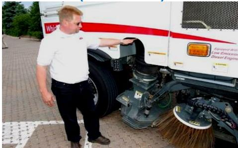
Vacuum street cleaners are the least common and most expensive. They apply a strong vacuum to a relatively narrow area that lifts particles both at and below the surface of the pavement. Vacuum sweepers have demonstrated their ability to suction 3 to 4 inches of gravel from PICP and can restore infiltration to some types of pavements that have been grossly neglected. (Hunt, NCSU-BAE)
