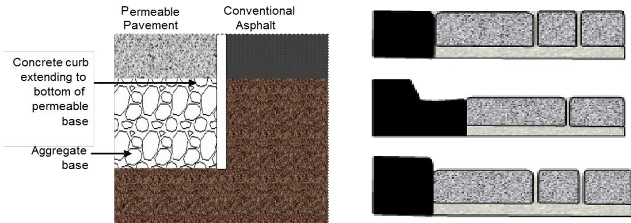
In addition to concrete edge restraints, an important consideration is the boundary between permeable and conventional pavement. At intersections between permeable pavement and conventional concrete, a geomembrane barrier should be provided to contain the stormwater under the permeable pavement and protect the base and subgrade under the conventional concrete. There should be a joint between the pavement surfaces for maintenance purposes.
