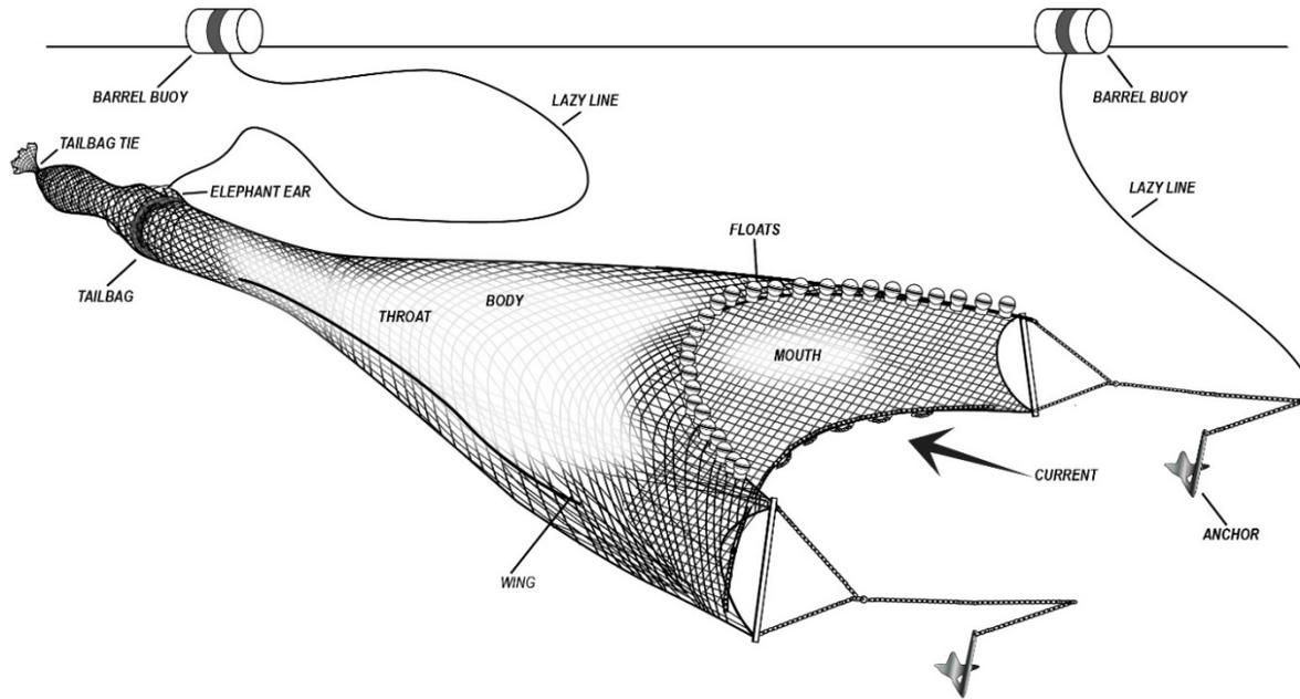
Figure 5. Schematic of channel net components.
