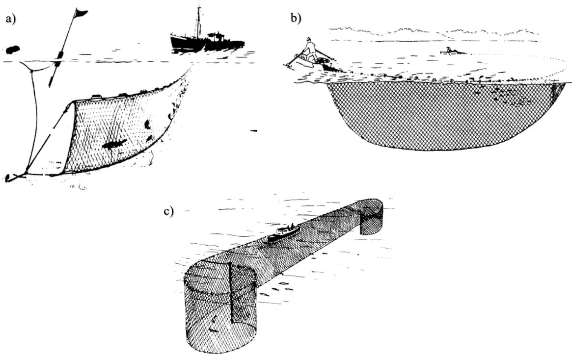
Figure 1. Illustrations of (a) set, (b) runaround, and (c) drift gill nets extracted from Steve et al. (2001).
