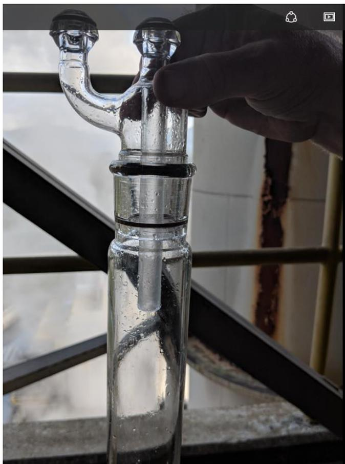
Picture 1 - Dropout Impinger
