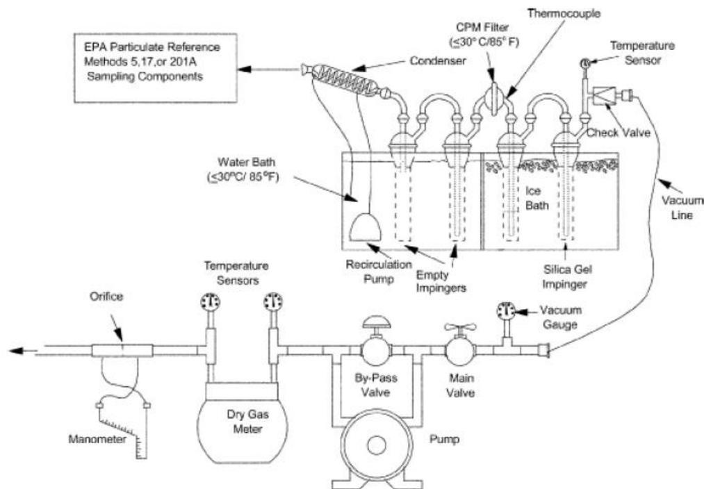
Figure 1 – Schematic of Condensable Particulate Sampling Train (Courtesy of the EPA)
