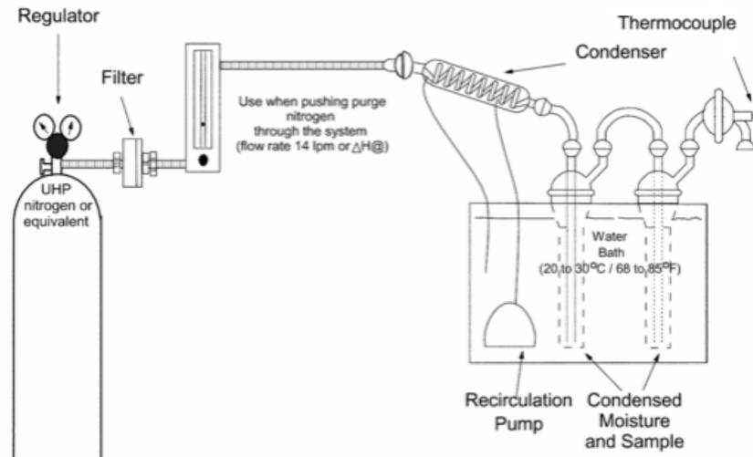
Figure 3 – Nitrogen Purge Setup (courtesy of the EPA)
