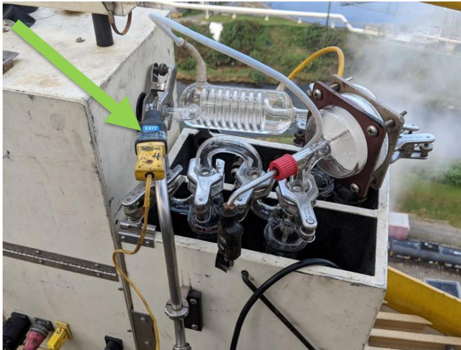
Picture 6 – Exit Impinger Thermocouple
