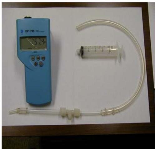
Figure 4.1 Pressure Test Setup
