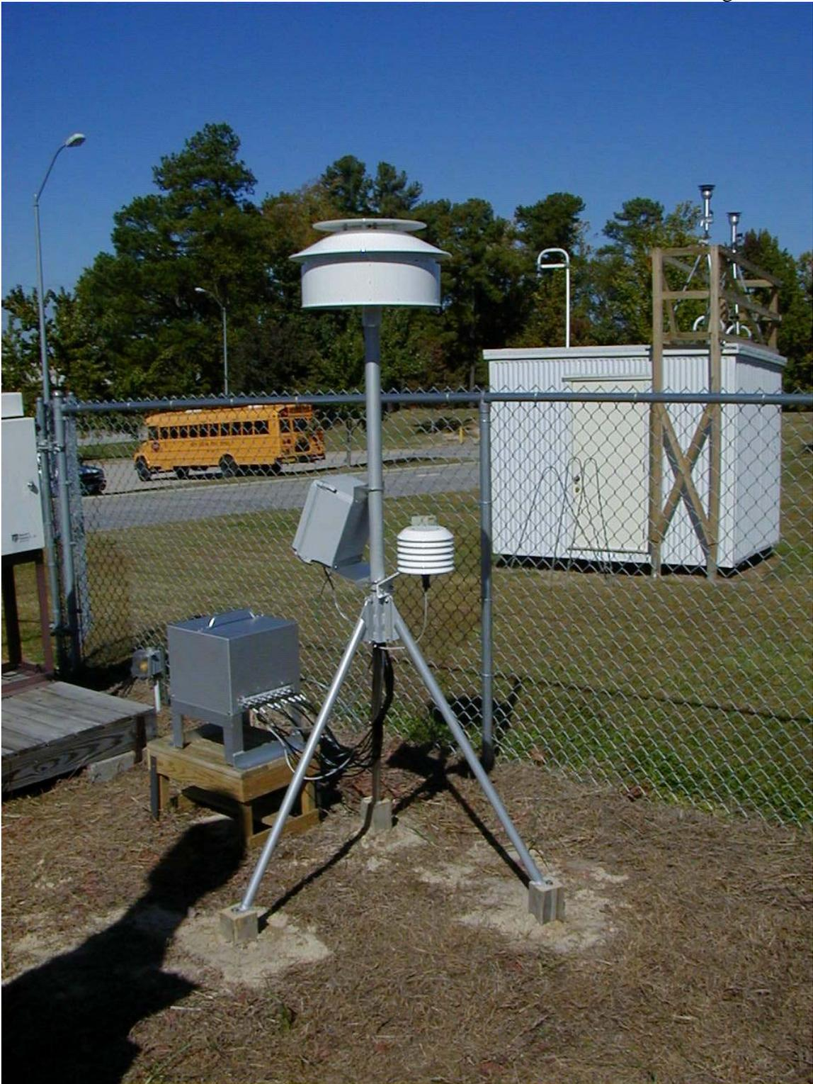
**Figure 2.45.1.1.1 Assembled SuperSASS Sampler**
