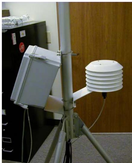
**Figure 2.45.1.2.3 Control Unit and Temperature Sensor Assembly**
