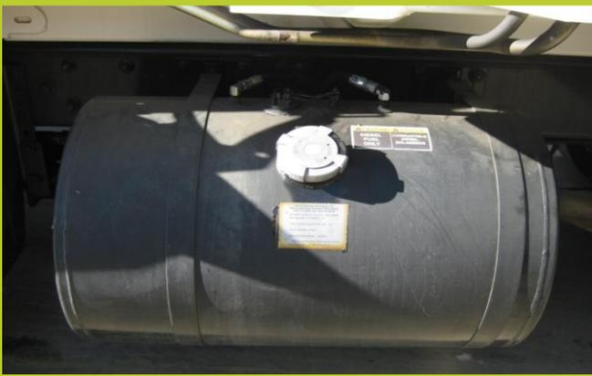
The CCC's tank (above) can hold 80 gallons of diesel fuel and is adjacent to where the DEF is added. Both trucks' Cummins ISC07-260 diesel engines are "Clean Idle" certified (below) because they generate very low NOx emissions when idling.
