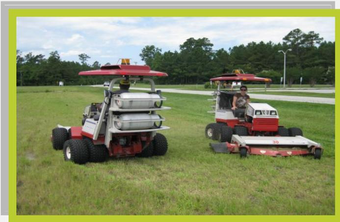
The propane mowers (above) come with two propane tanks for added convenience and to reduce refill time. When needed, the tanks are filled at the on-site filling station (below).
