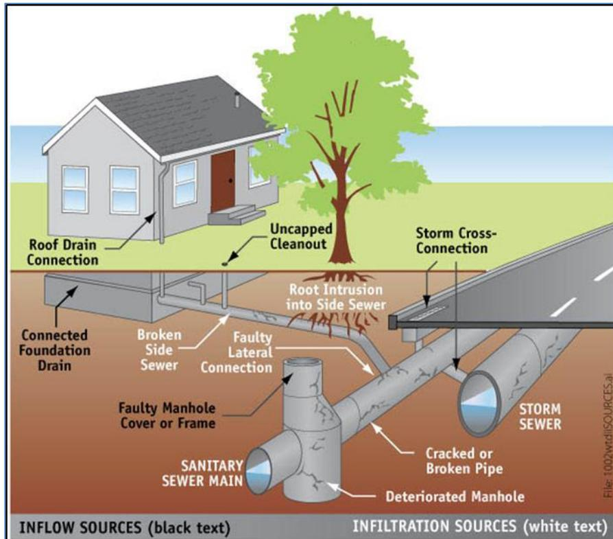
Figure 7.1. Example of inflow and infiltration (I & I) pathways.<sup>2</sup>
