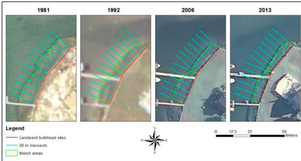
Figure 5.6. Time series of two bulkhead sites illustrating changes in marsh width, 1981-2013.<sup>100</sup>
