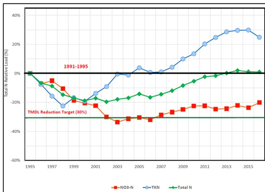
Figure 8.12. Flow-normalized nitrogen loads, Neuse River at Fort Barnwell Ambient Monitoring System (AMS) Station (Percent Change vs. 1991 to 1995).
