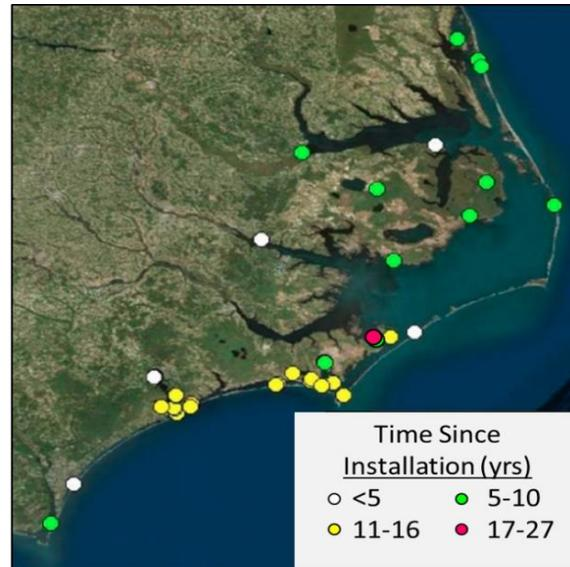
Figure 8.38. Surface elevation table (SET) locations in NC for monitoring long-term of elevation change.<sup>80</sup>
