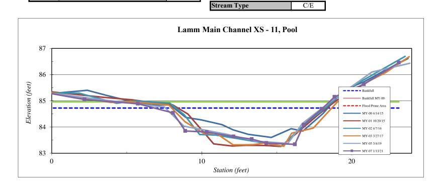
\*\*MY0-3 BHR were calculated using DMS method of "Dmax year x /Dmax year 0". MY5-7 were calculated using DMS method of area best fit. Some downcutting occurred just after asbuilt but has stabilized throughout monitoring period.
