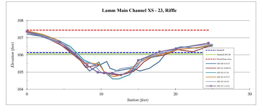
\*\*MY0-3 BHR were calculated using DMS method of "Dmax year x /Dmax year 0". MY5-7 were calculated using DMS method of area best fit. Overall channel area has remained constant. Sediment mobilization has resulted in minor downcutting, which has stabilized over the monitoring period. No problems are visible in this reach.
