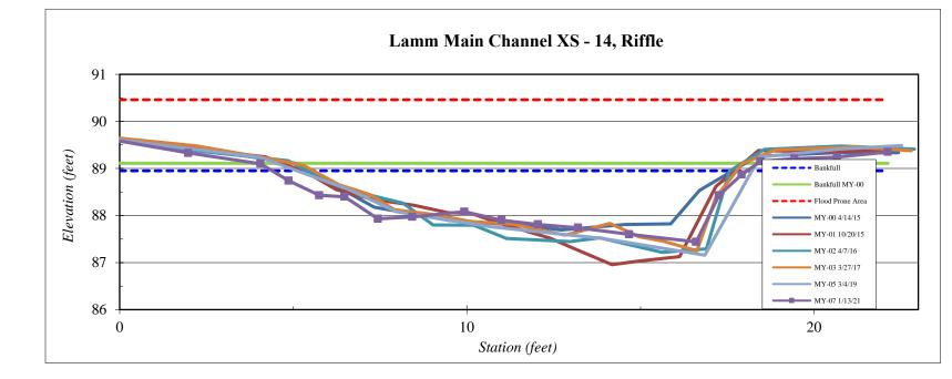
\*\*MY0-3 BHR were calculated using DMS method of "Dmax year x /Dmax year 0". MY5-7 were calculated using DMS method of area best fit. Channel constructed in lake bed. Unconsolidated materials are forming a new channel within the constructed channel. Depth is decreased between MY-0 and MY-01 and has stabilized since.
