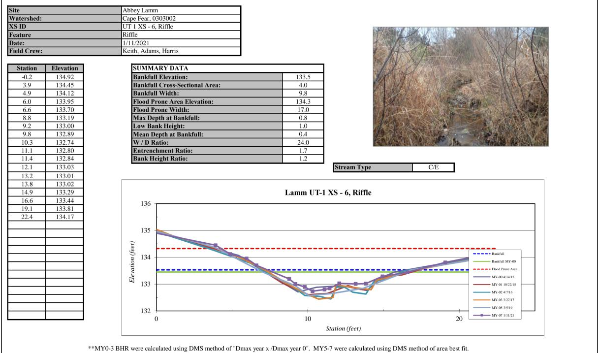
Overall channel area has remained constant. Sediment mobilization has resulted in minor downcutting, which has stabilized over the monitoring period. No problems are visible in this reach.
