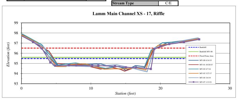
\*\*MY0-3 BHR were calculated using DMS method of "Dmax year x /Dmax year 0". MY5-7 were calculated using DMS method of area best fit. Enhancement Level II Reach. BHR varies through this reach; however, the reach is stable.
