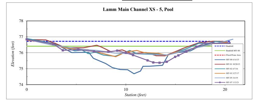
\*\*MY0-3 BHR were calculated using DMS method of "Dmax year x /Dmax year 0". MY5-7 were calculated using DMS method of area best fit. Sediment deposition in pool appears natural and is not expected to lead to instability.
