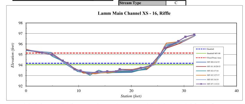
\*\*MY0-3 BHR were calculated using DMS method of "Dmax year x /Dmax year 0". MY5-7 were calculated using DMS method of area best fit. Enhancement Level II Reach. BHR varies through this reach; however, the reach is stable. Minor alterations in shallow channels may result in large discrepancies including elevated BHR.
