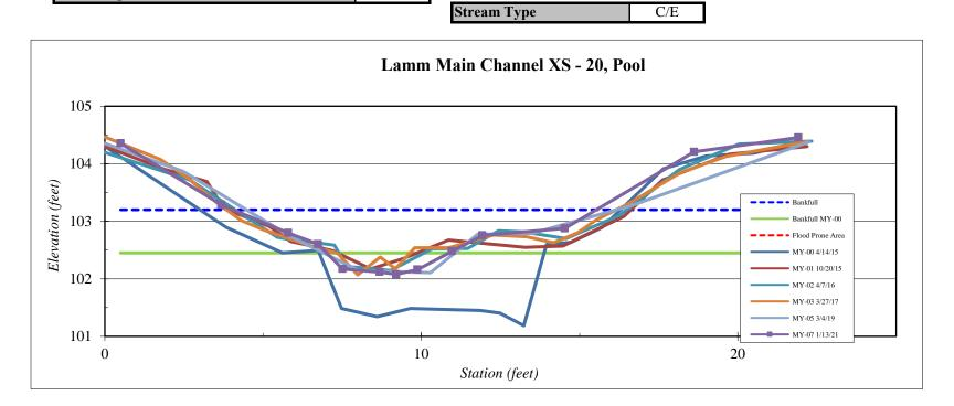
\*\*MY0-3 BHR were calculated using DMS method of "Dmax year x /Dmax year 0". MY5-7 were calculated using DMS method of area best fit. Sediment aggraded behind a bedrock sill after MY-0. Sediment has been stable throughout the monitoring period.
