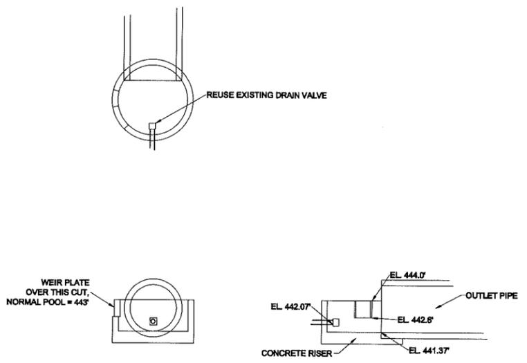
A STAINLESS STEEL PLATE WILL BE CONSTRUCTED AND INSTALLED BY THE ENGINEER, WITH A 1-FT VERTICALLY BY 1-FT HORIZONTALLY RECTANGULAR OPENING. THE INVERT OF THE WEIR PLATE WILL SET NORMAL POOL ELEVATION AT 443 FEET. THE FINAL MODIFICATIONS ARE TO PLUG THE EXISTING STANDPIPE WITH HYDRAULIC CEMENT AND CUT AROUND THE PERIMETER OF THE RISER AT THE ELEVATION SHOWN.
