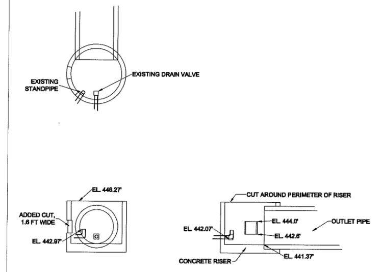
THE OUTLET STRUCTURE WILL BE MODIFIED AS SHOWN FOR USE DURING CONSTRUCTION. THE METAL TRASH GUARD WILL BE REMOVED. THE TOP PORTION OF THE RISER WILL BE CUT OFF AND REMOVED. A RECTANGULAR ORIFICE WILL BE CUT IN THE RISER AS SHOWN. A STONE SEDIMENT FILTER WILL BE CONSTRUCTED OVER THE ADDED ORIFICE AS IN DETAIL 7.2
