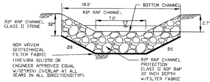
1 EMERGENCY SPILLWAY CHANNEL SECTION
