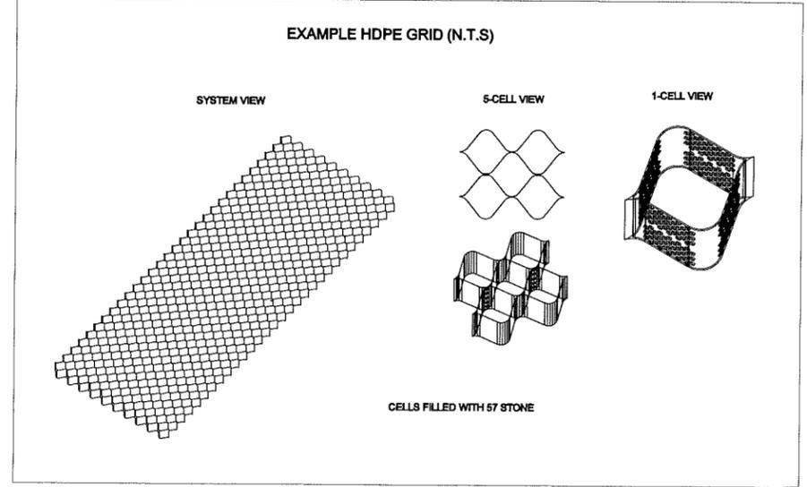
\*HDPE GRID MUST BE 6 INCHES TALL OR GREATER. GRID MUST BE PROPERLY SUPPORTED TO ALLOW H2O LOADING (AS DEFINED BY AASHTO), USING HIGH-STRENGTH FABRIC.
