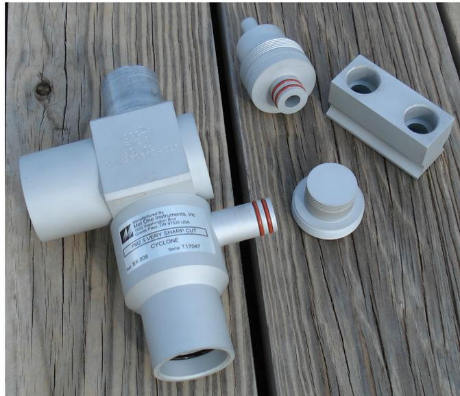
**Figure 28.** Disassembling the SCC for Cleaning
