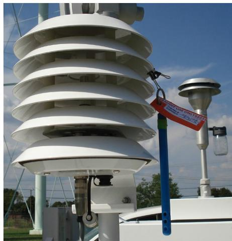
**Figure 23.** Proper Shaded Solar Shield Location
