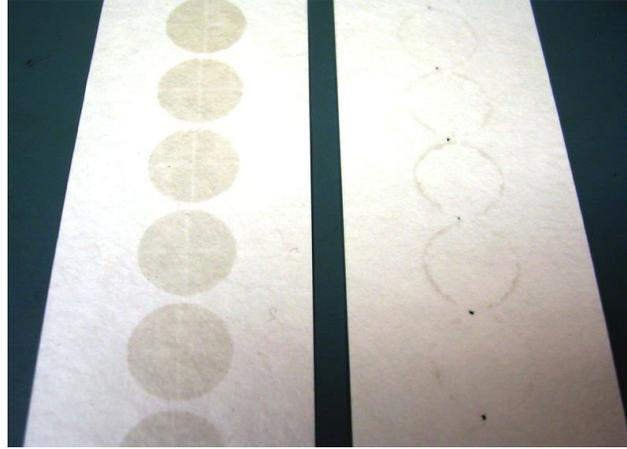
**Figure 30.** Hourly Filter Samples
