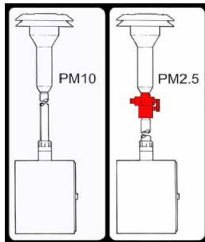
Figure 12. Door Label for Inlet Identification.
