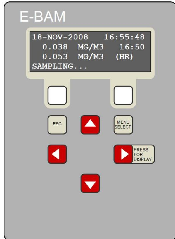
key is used to escape or exit out of a menu.
