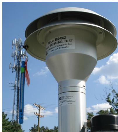
**Figure 18.** Proper Shaded Inlet Location
