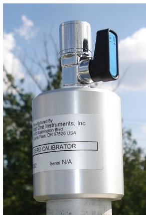
Figure 15. Leak Check Adapter
