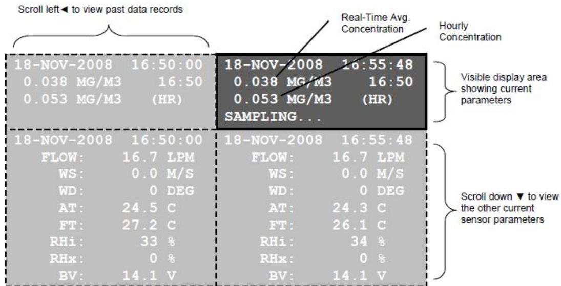
Figure 10. Main Sampling Screen Format.
