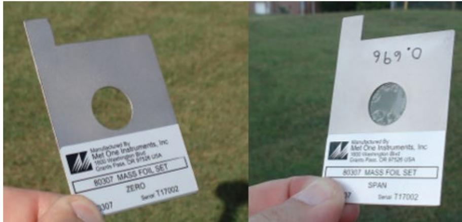
**Figure 25.** Zero and Span Foils.
