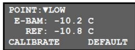
Figure 19. Temperature Sensor Calibration Menu.
