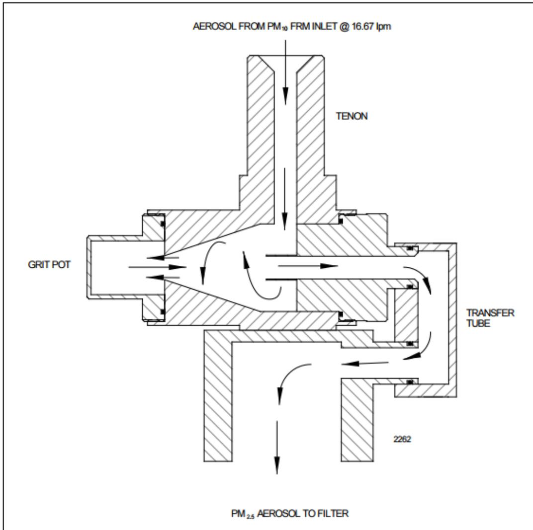
Figure 8. Operation of the SCC
