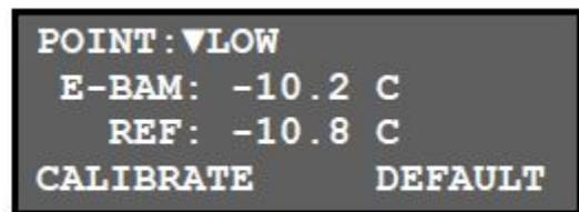
**Figure 24.** Temperature Sensor Calibration Menu.
