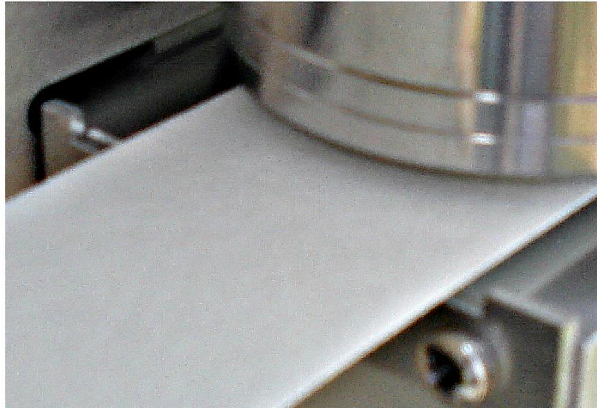
**Figure 14.** Tape Alignment Guide
