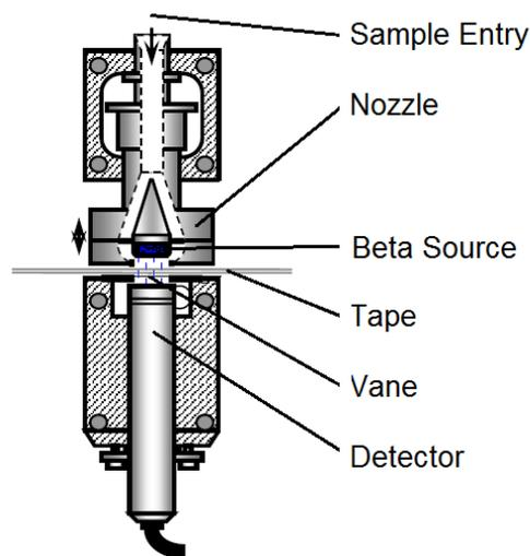
Figure 5. E-BAM Measurement System
