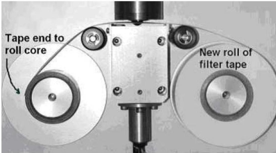
**Figure 13.** Tape Installation and Direction.
