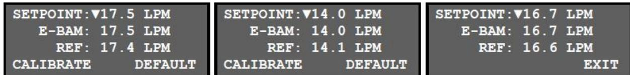
Figure 22. Sensor Calibration Menu for Flow.
