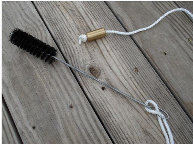
Figure 29. Pull Rope Assembly
