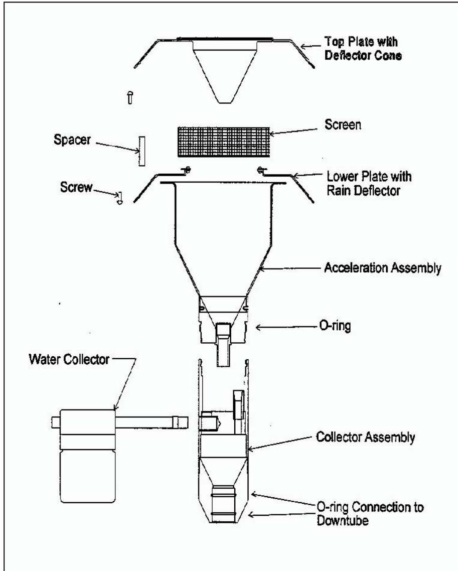
Figure 7. Exploded Cross-Sectional View of PM<sub>10</sub> Sampler Inlet Head
