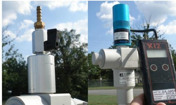
**Figure 21.** Flow Audit Adapter and FTS with Monometer.
