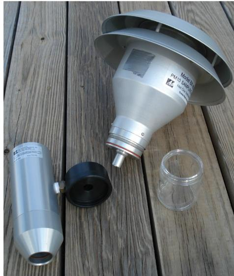
**Figure 26.** The PM<sub>10</sub> Inlet Components
