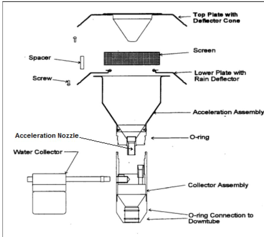
Figure 27. Exploded view PM-10 Inlet Assembly
