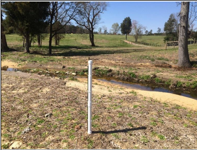
Reach 2, Crest Gauge at Station 38+75
