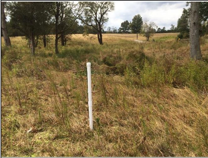
Reach 2, Crest Gauge at Station 38+75
