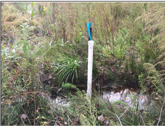
Reach 5, Flow Gauge #2 at Station 33+90
