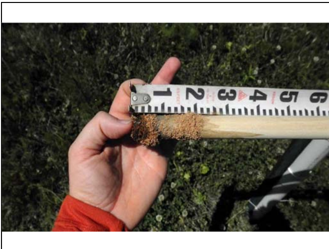
Reach 2: Crest Gauge, 0.21 ft on 5/2/17 (from 3.2" rain on 4/25/17, see associated spikes in flow gauge graphs)
