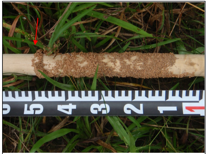
Close-up of overbank event of 1.49 ft from Hurricane Florence (photo: 10/10/18)
