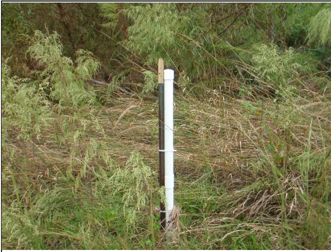
Crest Gauge on Reach 2 at Station 38+90
