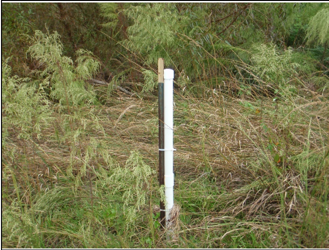
PP-31: Reach 2, Crest Gauge at Station 38+90
