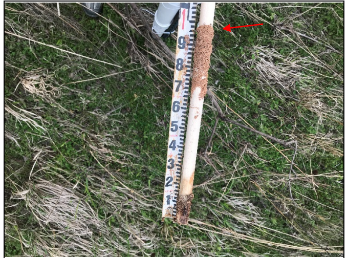
Overbank event of 0.97 ft (photo: 4/23/18)
