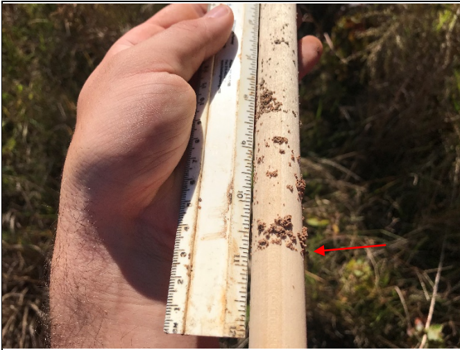
Overbank event of 0.89 ft on 4/19/19
