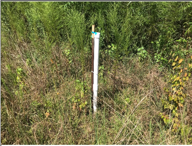
Crest Gauge on Reach R2 at Station 38+90
