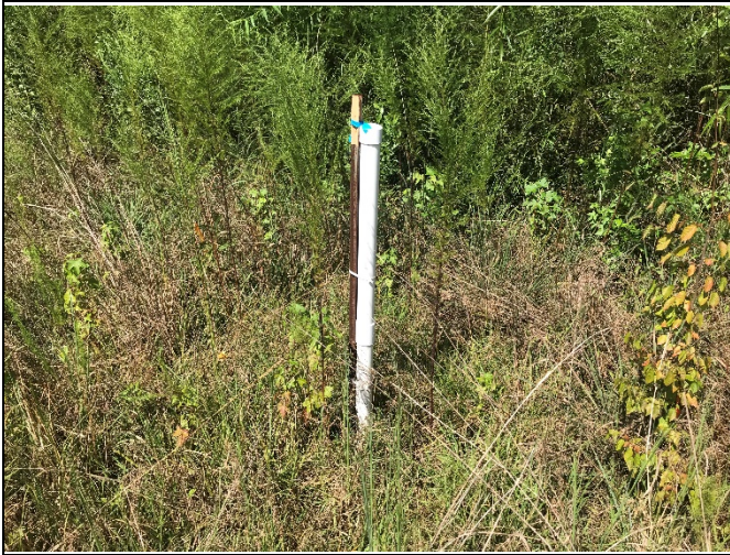
PP-31: Reach 2, Crest Gauge at Station 38+90
