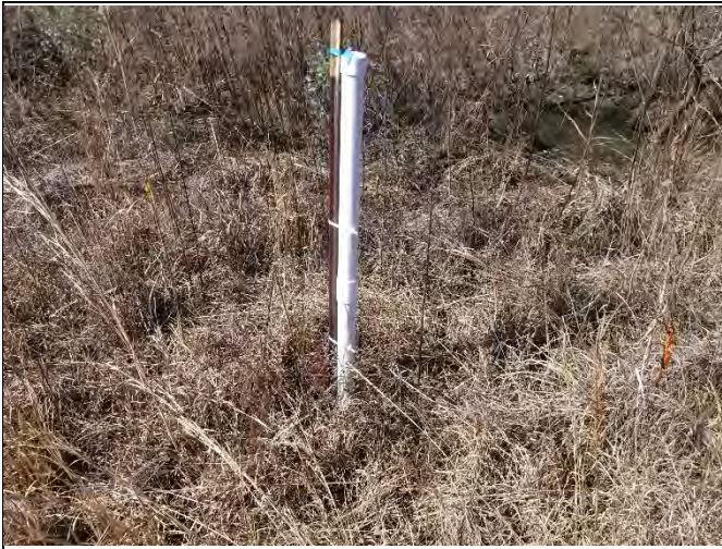
Crest Gauge on Reach R2 at Station 38+90 (photo from 2/14/20)
