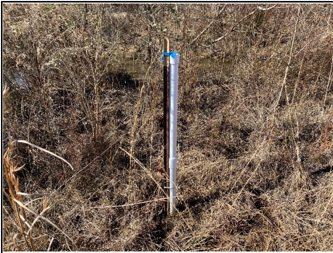
Crest Gauge on Reach R2 at Station 38+90 (photo from 2/18/21)
