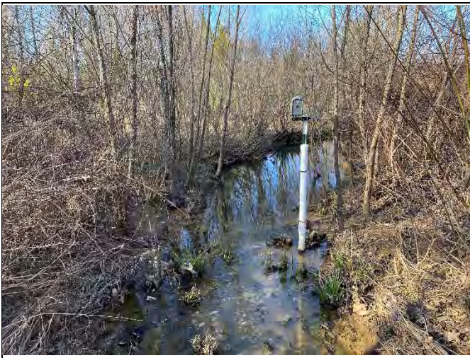
Flow Gauge in Reach UT4-R4b (photo 3/8/21) with flow camera attached at the top
