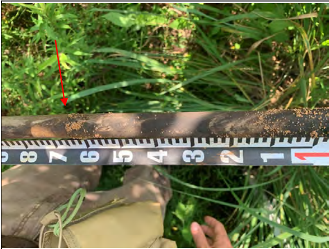
Crest Gauge Reach HC-R1: Close-up of gauge reading of 1.65' (photo from 7/22/21)
