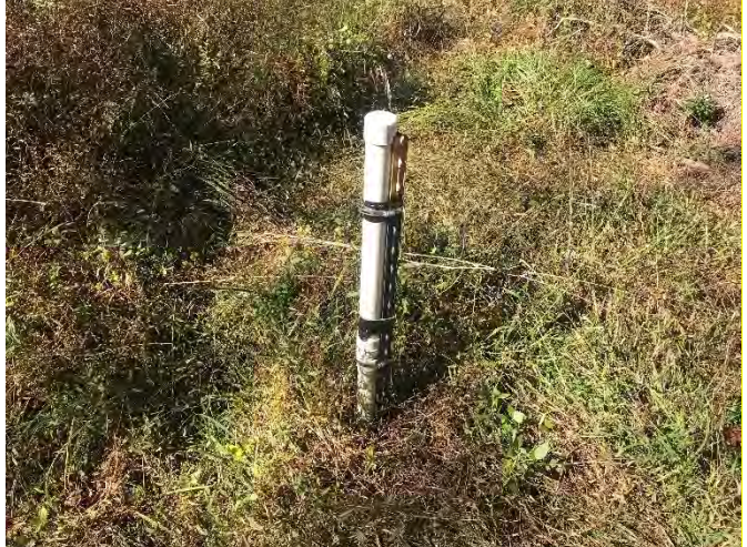
Manual Crest Gauge – Reach 1
