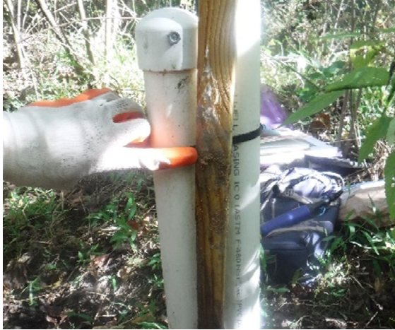
UT3 - Bankfull event recorded with Manual Crest Gage (Sta. 413+00) (10/19/2021)
