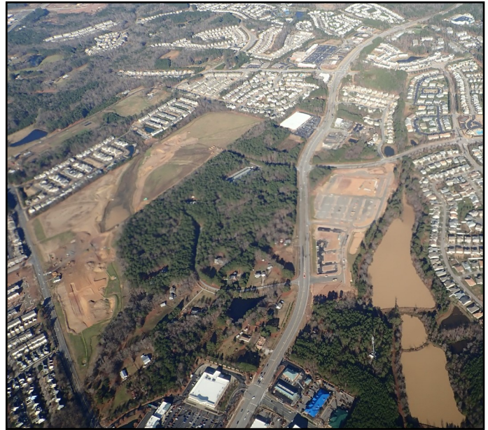
Aerial view of the impact of construction activities in the watershed of two ponds. Photo Credit: Rich McLaughlin.
