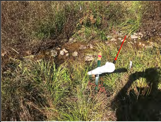
Continuous Stage Recorder #1 on UT5 (7/22/21)
