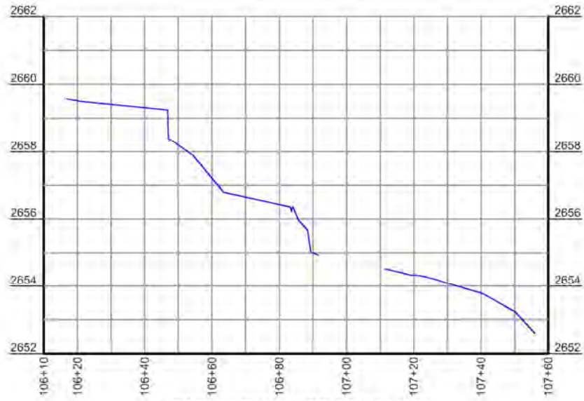
LONGITUDINAL PROFILE- UT1 HORIZONTAL SCALE: 1" = 20' FULL SIZE, 1" = 40' HALF SIZE VERTICAL SCALE: 1" = 2' FULL SIZE, 1" = 4' HALF SIZE
