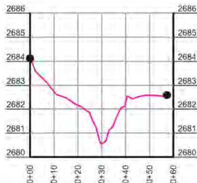
CROSS-SECTION #5 -UT TO CRAB CREEK HORIZONTAL SCALE: 1" = 20' FULL SIZE, 1" = 40' HALF SIZE VERTICAL SCALE: 1" = 2' FULL SIZE, 1" = 4' HALF SIZE
