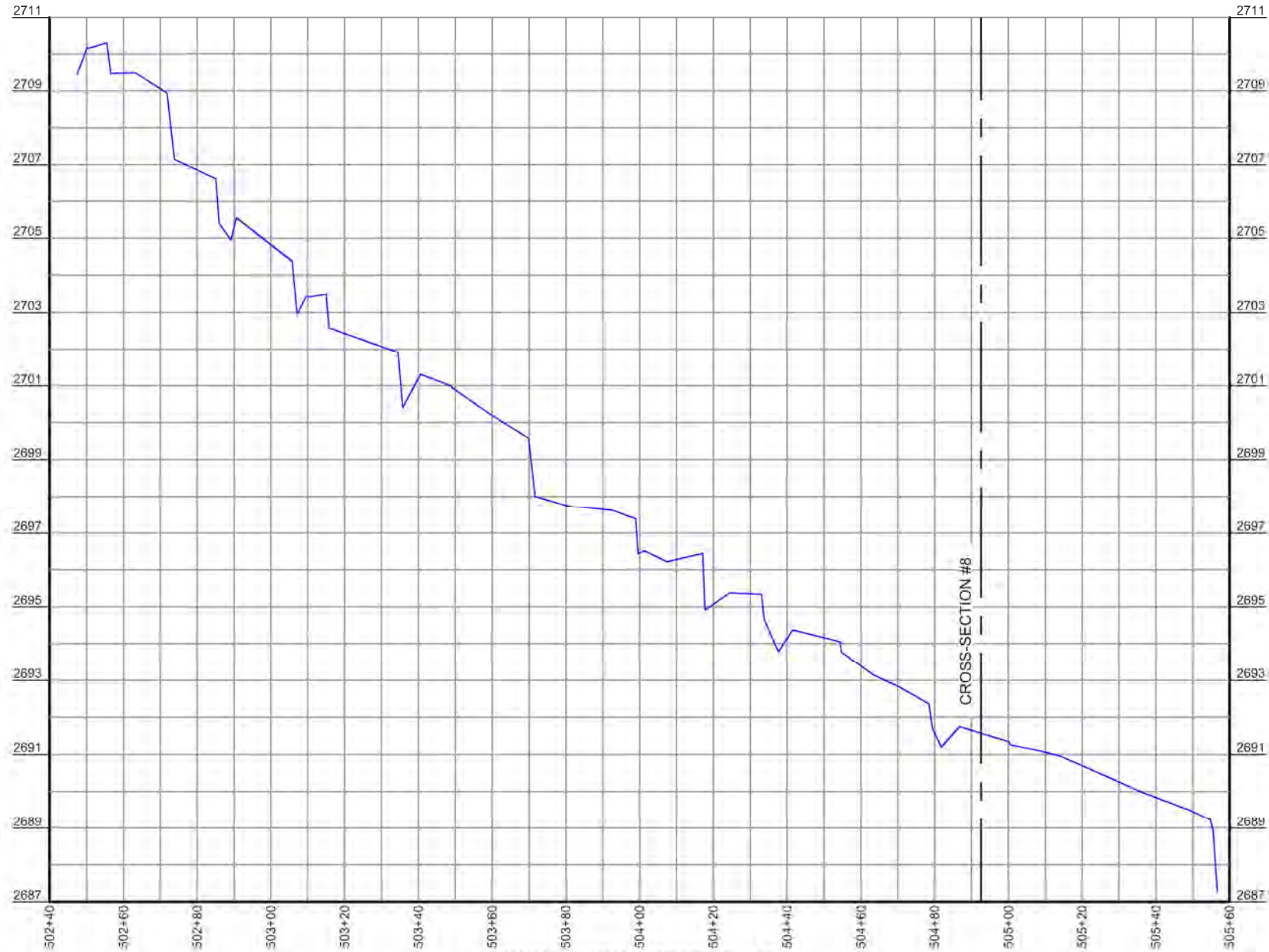
LONGITUDINAL PROFILE- UT5 HORIZONTAL SCALE: 1" = 20' FULL SIZE, 1" = 40' HALF SIZE VERTICAL SCALE: 1" = 2' FULL SIZE, 1" = 4' HALF SIZE
