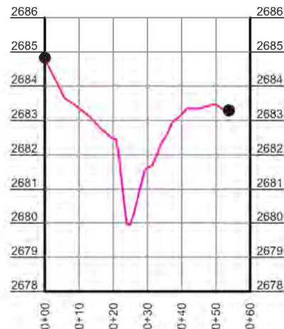
CROSS-SECTION #4 -UT TO CRAB CREEK HORIZONTAL SCALE: 1" = 20' FULL SIZE, 1" = 40' HALF SIZE VERTICAL SCALE: 1" = 2' FULL SIZE, 1" = 4' HALF SIZE
