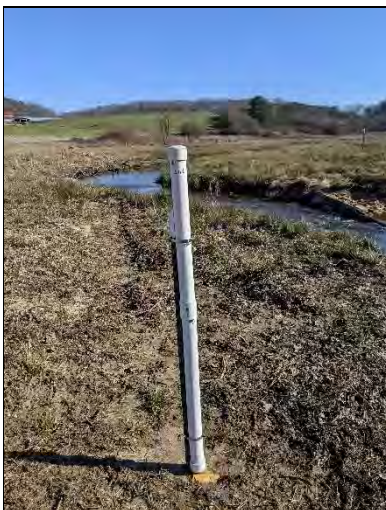
Crest Gauge 1: R1: 1-27-2022
