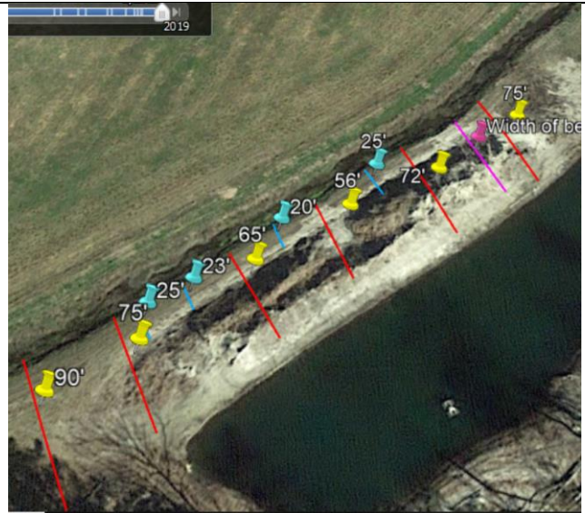
2019 imagery showing pond footprint, recent removal of trees, & excavated material/berm pile located in Zone 1 and some of Zone 2 of riparian buffer. Approximate measurements taken in feet from top of bank along stream to previous (before clearing) edge of forest (Red lines) & approximate measurements in feet taken from top of bank along stream to edge of berm pile (Blue lines).
