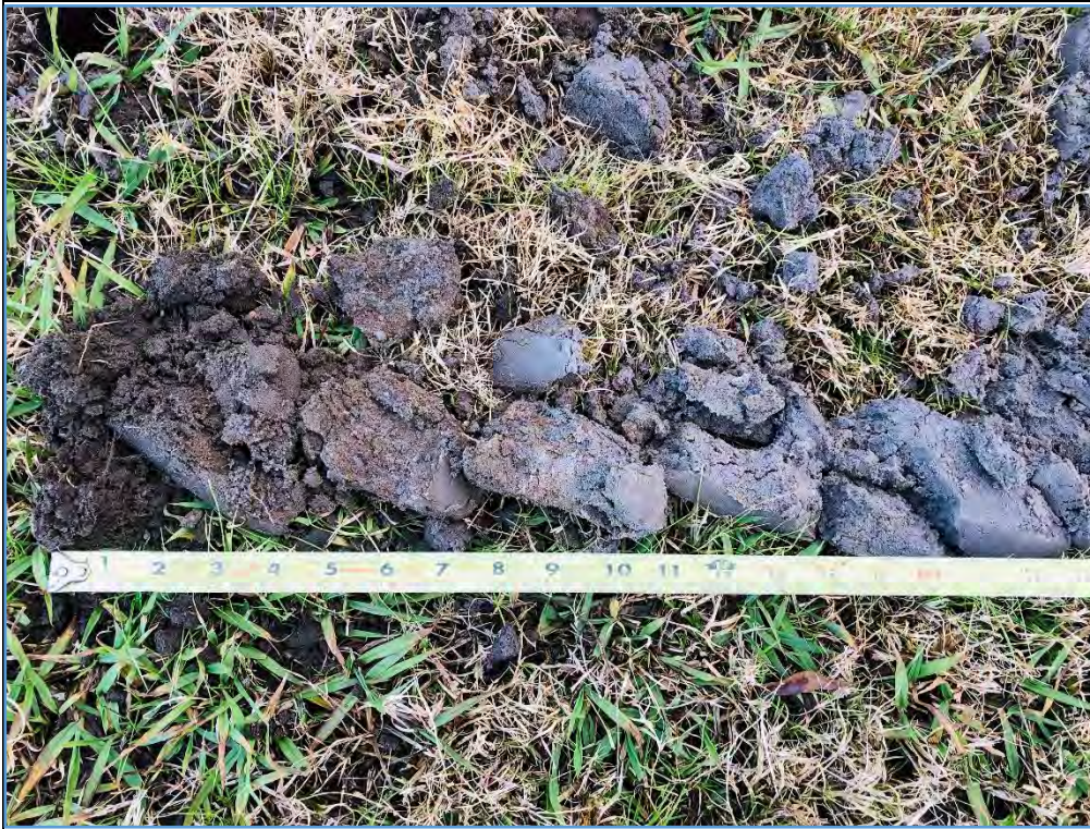
1. Hydric profile. Meets the A11 Depleted Below Dark Surface , F3-Depleted Matrix , and F6-Redox Dark Surface indicators. SB#60.
